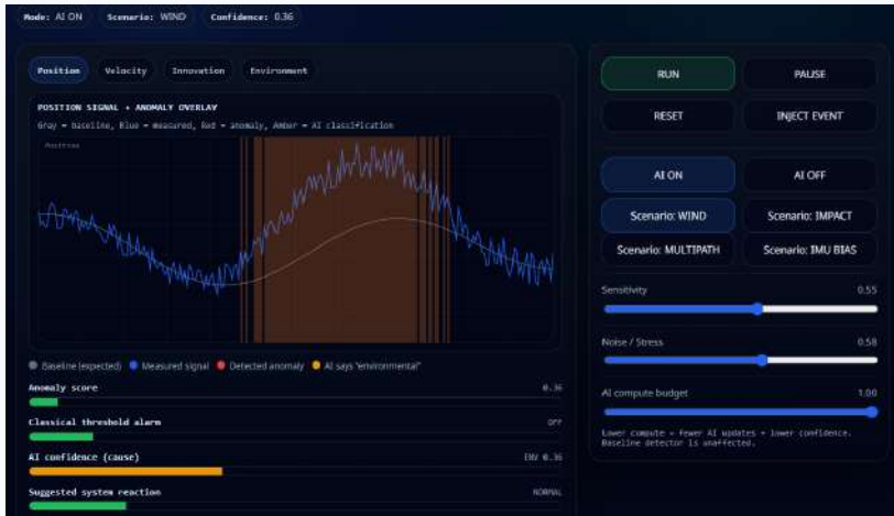
Figure 15.2: Anomaly Classification and Confidence. Classification confidence represents belief over anomaly cause rather than correctness. Overconfidence is mitigated by retaining residual statistics and estimator coherence checks as primary signals.
